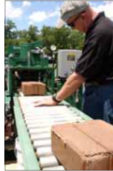
Finished bricks made from ordinary soil roll from TerraBuilt's "Green Machine." See the "Green Machine" in action at the 2007 Piedmont Alternative Energy Expo. Photo by Lili Duvall.
